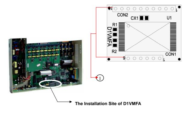
1. Connect to the [F2A] ~ [F5A] and [F3B] ~ [F5B] positions where upon the D1VMCA.
