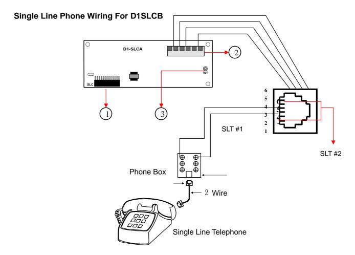
Figure 23. SLT Station Wiring on D1SLCB
