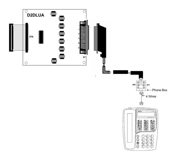
Figure 21. Digital Key Station Wiring on D2DLUA
