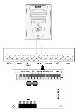
Figure 24. Door Phone Wiring on D1MFCA
