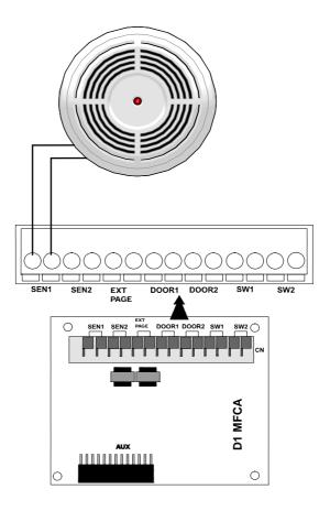
Figure 25. External Sensor Wiring on D1MFCA
