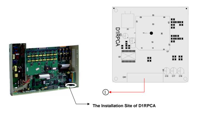
1. RPC: 26-Pin Connector to connect to [RPC] position where upon the D2MBUB.
