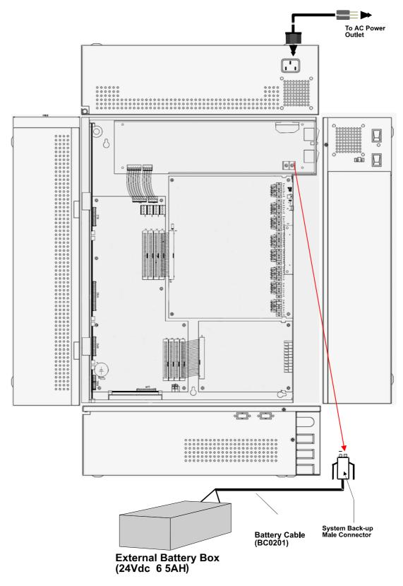
**NOTE.** AC Power input to the system can be either 115VAC or 230VAC. The system can detect the input voltage automatically.
