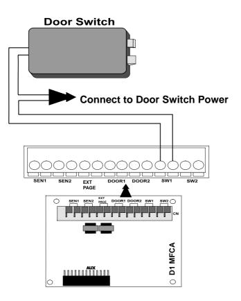
Figure 26. Door Switch Wiring on D1MFCA
