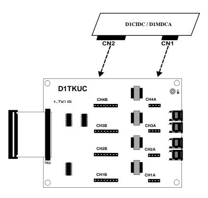
Figure 20. Metering Pulse Detection Card Installation
