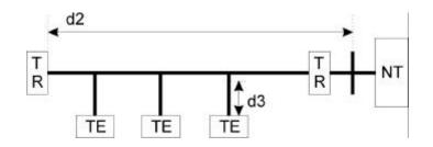
d2: 100m ~ 200m; Length limitation by round trip delay 10us to 14us, not by attenuation.
