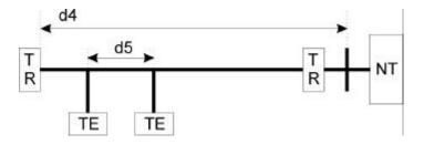
d4: 500m ~ 800m; Length limitation by round trip delay 10us to 14us, not by attenuation. d5:  $25m \sim 50m$ ; Length limitation between TE's by differential round trip delay of 2us.
