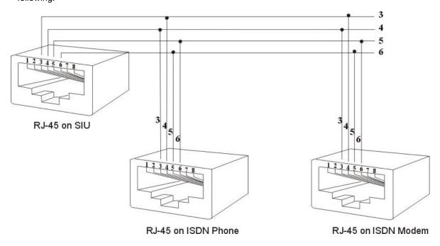
• Bus Configurations on the S/T Interface: *Point to Point:*
