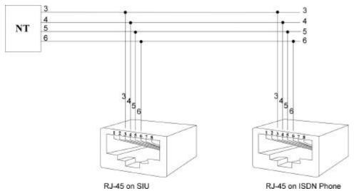
S-Interface Connection: If the user has programmed the ISDN interface of SIU to a S-Interface, the wiring should be as the following:
