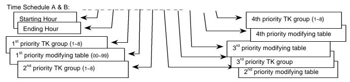
Time schedule C does not have the Starting/Ending hour setting. Only priority trunk groups and modifying tables need to be assigned. . If only 1 Time Zone is to be used then use Time Schedule C which will automatically cover 24 hours if Schedule A and B are blank.
