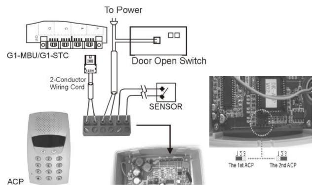
CAUTION !: Avoid shorting Tip and Ring together. It may damage the G1-MBU or G1-STC board.
