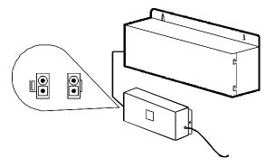
If you are installing an optional Battery Backup (BBOX1), make certain that there is adequate room for its installation. Make certain that the Battery Backup is mounted close enough to the Power Supply that the interconnecting cable between the Battery Backup and the Power Supply can connect. **Do Not Connect the Battery Backup at this time!**
