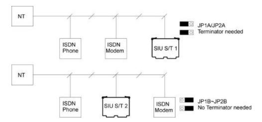
Adjust 8K/256K jumper on SIU for the ISDN line. Adjust it to 8K position for most ISDN lines.
