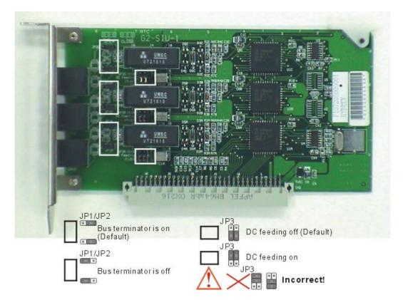
**JP3(A,B,C):** DC feeding jumper. Default is no DC output. If the internal ISDN device does not offer local power and need DC feeding to work. The related jumper of this internal ISDN interface needs to be set to "on".
