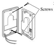
**2.** Attach the base cover to a wall using 2 screws.
