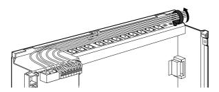
**4.** To remove the rivet, use a screw driver as shown below.
