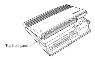
**3.** After cutting the areas, be sure to cut off any excess plastic in order to make the surface smooth. Please refer to installing the KX-TA30877.
