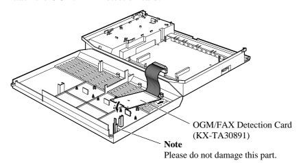
**4.** Insert the flat cables to the card connector.
